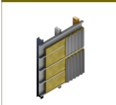
Profiled wall with cassette structure | see page 70
